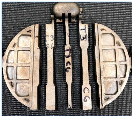
Figure 5 – One of the HPDC coasters after wire EDM cutting showed where the tensile coupons were extracted. The area in the center was saved for hardness measurements and microstructure analysis.
