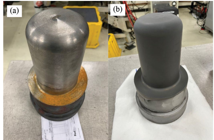
Figure 11 – Photos showing the in-plant trial punch: (a) before and (b) after depositing the self-lubricating nanocomposite coating.
