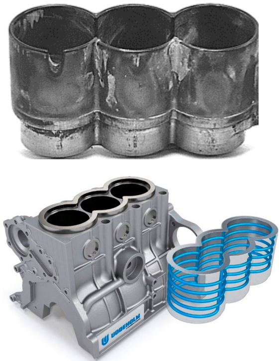
Figure 1 - Soldering formation on water jacket inserts and conforming cooling design.
