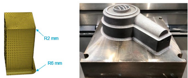
Figure 3 - Printed geometry with design recommendations.
