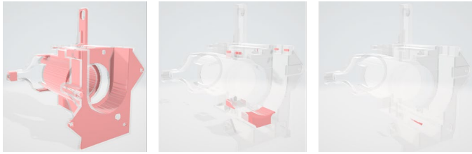
Figure 11 – The thick selection in depth a) 0.76 mm, b) 3.04 mm and c) 6.08 mm.
