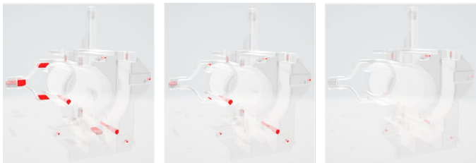
Figure 13 – The thin die selection in depth a) 6.08 mm, b) 3.04 mm and c) 0.76 mm.
