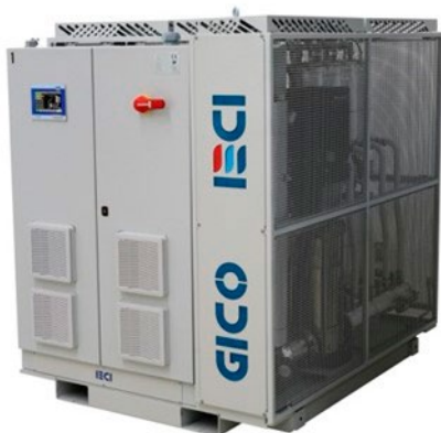
Figure 2 - Photo of a GIGATHERMO® Compact (GICO) unit, 320°F, with flow rate of 127 gpm @ 8 bar, 144 kW heating and 600 kW cooling power, it can feed up to 30 different circuits.
