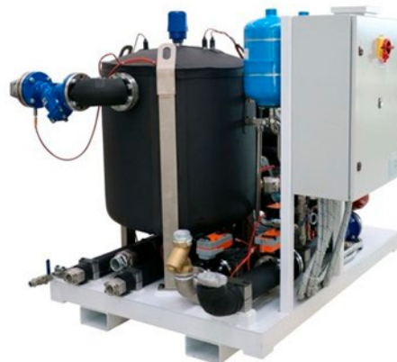
Figure 3 - Model of a HYPERCOOLING system with pressurization pump of up to 400 l/min @ 16 bar with variable speed. Pressure, flow and temperature sensors on each circuit. Thermal power (btu/h) and exchanged heat (btu) calculation. Integrated leak test with compressed air with independent detection on each circuit.
