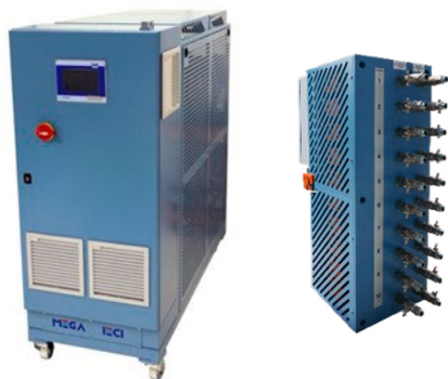
Figure 1 - Photo of a MEGATHERMO® TCU unit, 320°F, with flow rate of 100gpm, 54 kW heating and 300 kW cooling power and a Pioneer® manifold with 10 proportional circuits.
