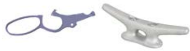
Figure 3 – Two steel parts to be die cast, new tooling is being constructed, the steel die cast process will be developed for each of these castings
