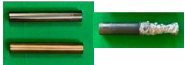
Figure 5 – Shows the coated and uncoated copper cores. The Figure to the right show the dissolution of an un-coated copper core after two minutes in molten aluminum
