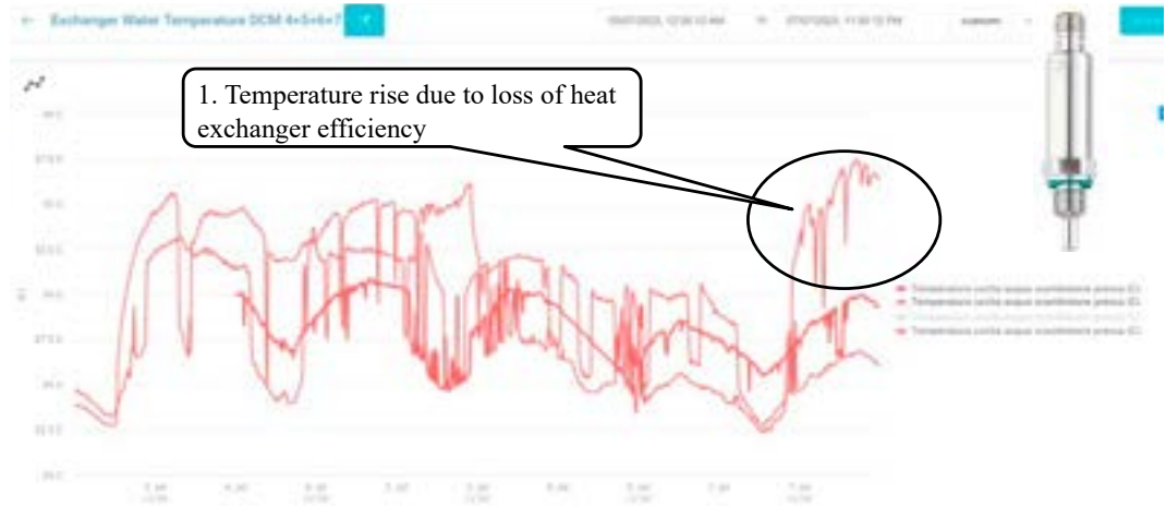
Figure 5 - Measuring the efficiency of the heat exchanger.
