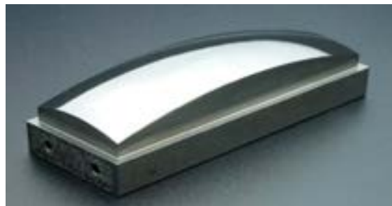
Figure 9 - Polishing-sample (H13; heat-treated).
