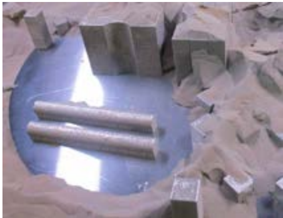
Figure 4 - Oxidation-free powder due to minimized oxygen level.
