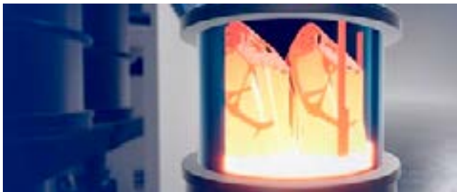
Figure 1 – TP500's build and supply cylinders / schematic view into build cylinder with preheated substrate plate.
